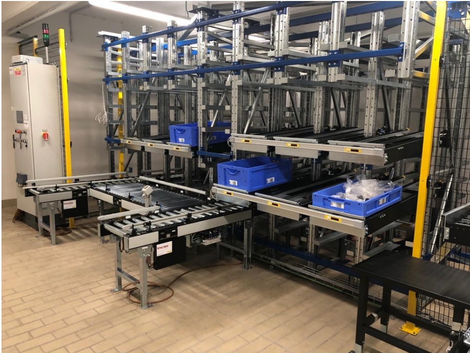
Figure E.2. The AS/RS with the two working stations.
