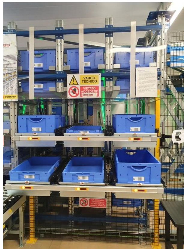
Figure E.3. Picking station with pick-to-light system.
