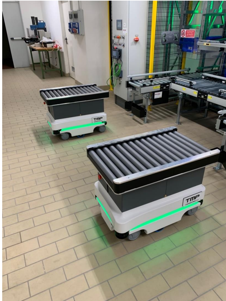
Figure E.1. The two AGVs connected to the AS/RS.
