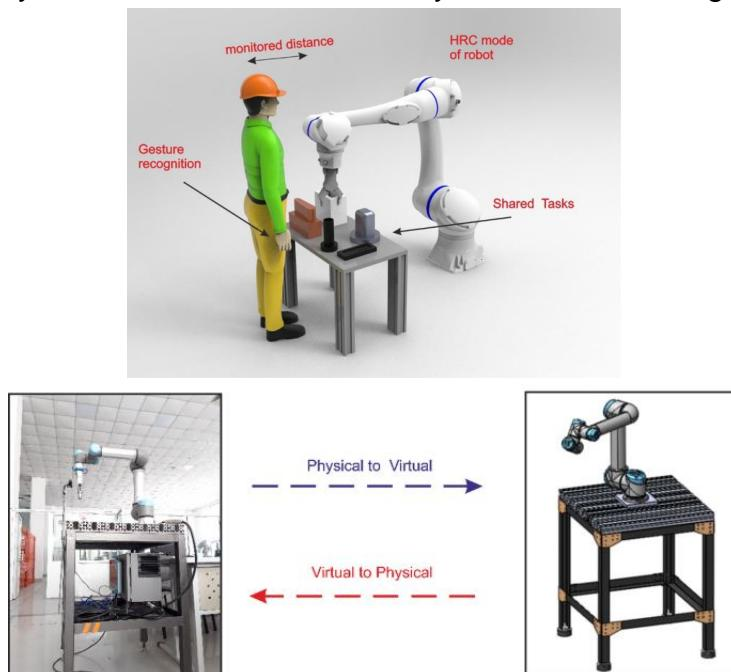
POLITO developed a methodology to establish a traceable digital twin of a robotic arm collaborative robot (cobot). The digital twin leverages a machine vision system, calibrated by laser tracker, to continuously monitor its position and compensate for motion error. The work allowed to evaluate the positioning uncertainty of the cobot reducing the positioning error uncertainty from 2 mm to 0.2 mm.
