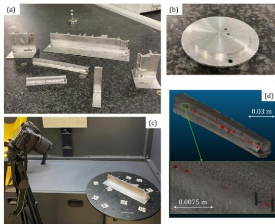
**Politecnico di Torino (POLITO)** developed a methodology for establishing traceability and evaluating measurement uncertainty of machine vision systems for the automatic detection of surface defects. The methodology was applied to a case study aimed at inspecting the surface quality of corner welds in gas metal arc welding of cast and rolled aluminum components for automotive. The work was presented at the 74th General Assembly of the International Academy for Production Engineering (CIRP).
